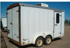
1996 Avenger enclosed trailer, 14'X 7' tandem axle with partition in the middle, front portion 8'X 7', back portion 5'5" X 7'
